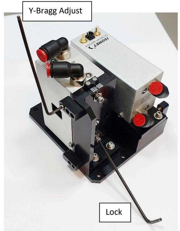
*The coolant and RF connections can resist Bragg angle adjustment. It may be necessary to assist the AOD rotation with a little hand pressure on the AOD case. This is most likely needed for counter-clockwise rotation of the Bragg adjuster.*
